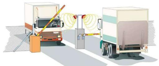
Radio Frequency Identification (RFID) devices consist of tags and readers that assist in the tracking of goods and vehicles. Tags are the devices that give identity to the vehicle and work like a wireless name plate. It transmits it identity to readers which are placed at strategic locations like entry/exit of a premise, highway, weighing bridge, parking lots and others.
