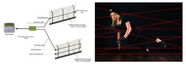
It is an invisible and active perimeter protection system. It can be used for indoor applications also. A transmitter consisting of an infra red source emits an invisible beam and that is made into a sharp pencil beam for rectilinear propagation by using a lens arrangement and the pencil beam is received by a photo electric detector after being focussed by lens arrangement at the receiver placed at about 70 - 100 ft. outdoor or 20-30 ft in indoor application. Transmitter and
